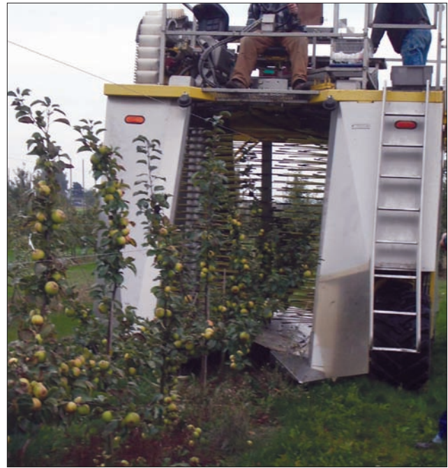
Figure 22. Trial of machine harvesting cider apples (variety Brown Snout) with a raspberry picker.
