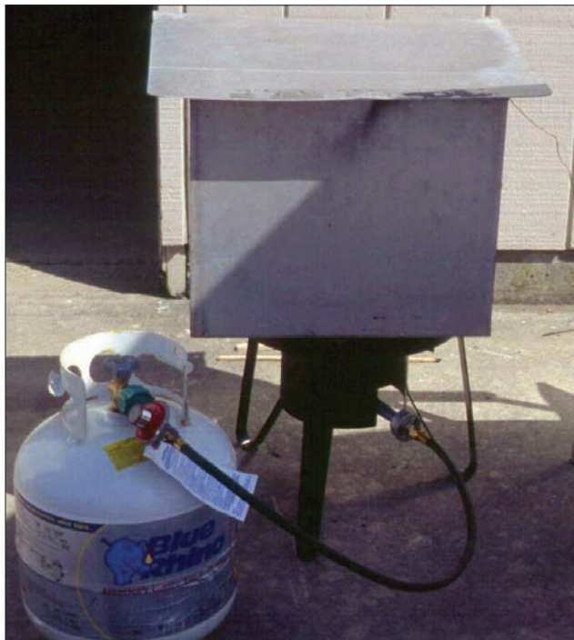
Figure 17. Home pasteurization. For small-scale operations, a propane-heated water bath with accurate temperature control can be used (left). Be sure to wear protective clothing (right) during this procedure.
