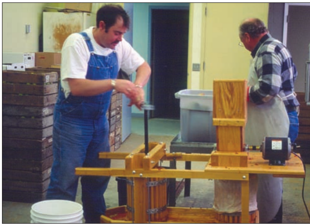
Figure 8. Small-batch home cider combined mill and press.
