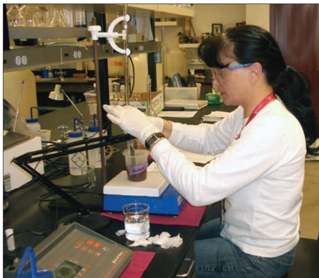
Figure 11. Titration method for determining pH and titrateable acid in apple juice.
