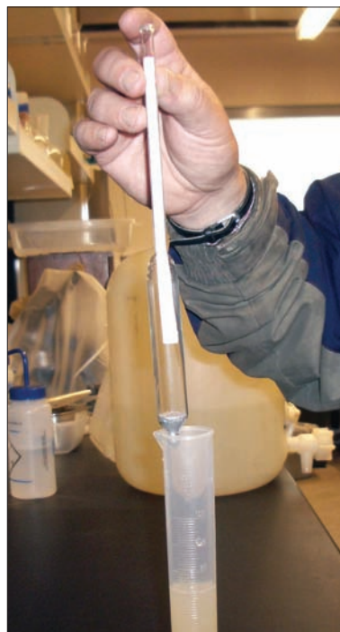
Figure 12. Using a hydrometer to measure the specific gravity of a juice sample.
